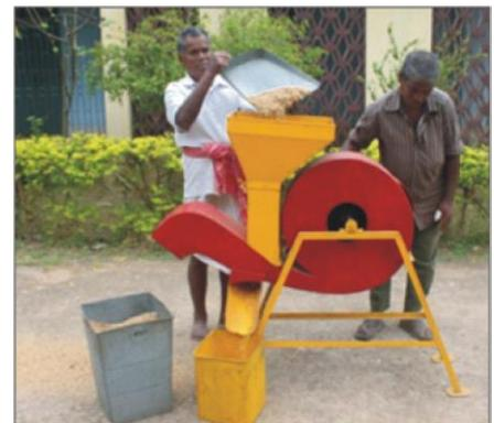
**CRRRI Power Rice Winnowing cum Cleaner** is a power operated machine to clean threshed paddy crop. Its capacity is 500 kg/hr of clean paddy, having cleaning efficiency of 99%. Cost of the machine is Rs.1 8,000.
