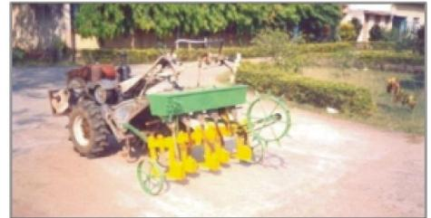
**CRRRI Power tiller operated seed drill for rice and Groundnut** is a five row seed drill having plastic wheels with grooves on its periphery as seed metering mechanism. It is suitable for dry sowing rice and groundnut. Its row to row spacing is 25 cm. The cost of the seed drill is Rs. 22,000. The field capacity of 0.14 and 0.15 hectare per hour and cost of planting of Rs. 1240 per hectare and Rs. 1200 per hectare was observed for rice and groundnut, respectively.
