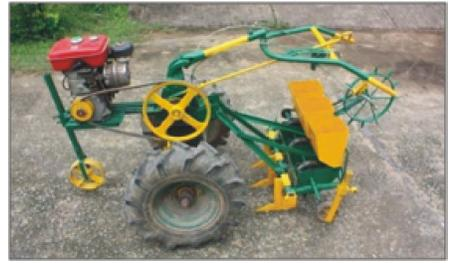
**CRRRI Power tiller operated seed drill for rice and pulse** is a five row seed drill having fluted roller type seed metering mechanism. It is suitable for dry sowing of rice, wheat, green gram, and black gram etc. Its field capacity is 0.14 hectare per hour. Its unit cost is Rs. 20,000.
