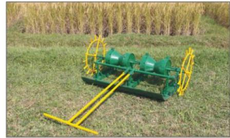
**CRRRI Six row manual drum seeder (Cylindrical shape)** is suitable for sowing of sprouted paddy seed in puddled field at row spacing of 20 cm. Its field capacity is 0.037-0.04 hectare per hour. Its unit cost is Rs. 6500. It reduced seed rate by 35-40% as compared to broadcast seeding and reduced weeding cost about 55%.
