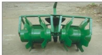
**CRR I drum type disc harrow** is a bullock drawn implement used for puddling. It has two gang with 3 plane disc mounted over each hollow drum. Its field's capacity is 0.4 hectare per hour. Two operations of float-harrow are sufficient to create field conditions ready for transplanting the seedlings. Its unit cost is Rs. 20,000. The puddling time is decreased from 42 hours which is required in case of indigenous plough to 11 hours.
