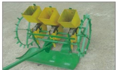
**CRRRI Four row manual drawn seeder (hyperboloid shape)** is suitable for sowing sprouted paddy seed in puddled field at row spacing of 20 cm. Its field capacity is 0.030-0.034 hectare per hour. Sowing with drum seeder reduced seed rate by 60 - 65% as compared to broadcast seeding and reduced weeding cost about 65%. Its unit cost is Rs. 4500.
