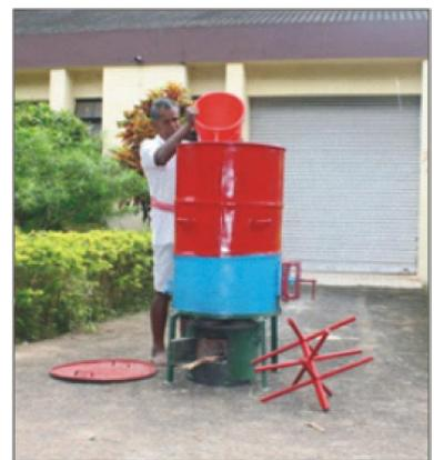
**CRRRI Mechanical Rice Dryer** is a variable capacity batch dryer of 125-500 kg capacity. Both raw and parboiled paddy can be dried in this dryer. Drying is accomplished on thin layer principle. The air temperature can be maintained at  $40 \pm 2$  OC throughout the drying period. Paddy at moisture content of 20% was dried to 14% in 6-7 hrs using 10 kg of coal in the furnace. Cost of the dryer is Rs. 50,000.
