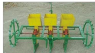
**CRRRI Three row self propelled hill seeder** is a three row seeder suitable for dry hill seeding of rice. It has 3.5 H.P. petrol start kerosene driven engine as a source of power. Its row to row spacing is 20 cm. Its field capacity is 0.1 hectare per hour. Its unit cost is Rs. 50,000.
