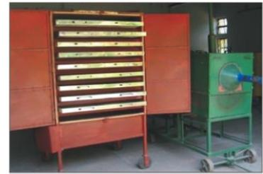
**CRRRI Domestic Solar Dryer** is a cabinet type domestic solar dryer to dry 0.5 - 1 kg food material. The dryer is rectangular in shape. The top glazing is of 4 mm plane glass. The dryer is placed on a stand inclined at an angle of 30° to the horizontal. A sliding type loading tray enters from the top end of the dryer. Cost of the dryer is Rs. 1,500.
