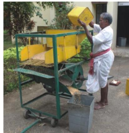
**CRRRI Power Rice Seed Cleaner** is a power operated machine to clean threshed paddy crop for seed purpose. Its capacity is around 8 q/hr of clean paddy, having cleaning efficiency of 99%. Cost of the machine is Rs. 30,000.
