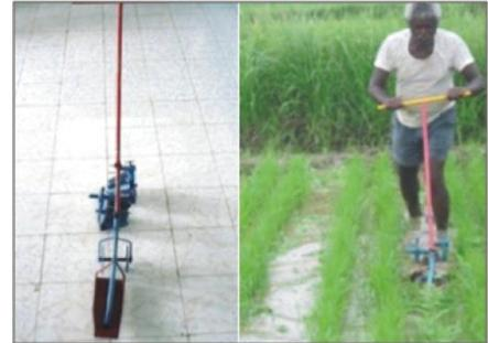
**CRRRI wheel finger weeder** is suitable for weeding of row crops like upland rice, jute, maize and vegetable crops. It is manual pull and push type weeder. The weeder consists of a frame, a wheel, a handle and five no of curved fingers. The spacing between fingers is adjustable. As the operator moves the handle to and fro the fingers push into the soil and loosen it and the weeds get uprooted. Field capacity of this implement is 0.022-0.025 hectare per hour and its unit cost is Rs. 600.
