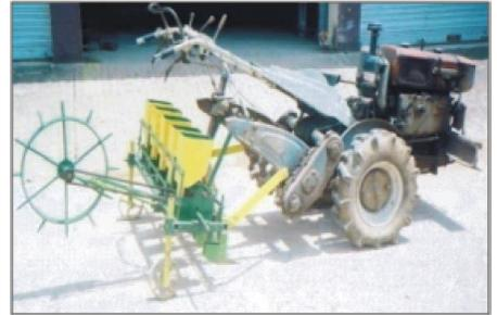
**CRRRI Ten row tractor drawn seed drill** is a ten row seed drill and suitable for seeding in dry field. The field capacity of the seed drill is 0.8 hectare per hour. Row to row distance can be adjusted. The unit cost of machine is Rs. 50000. It saved 70% time and 55% labour cost and weeding cost as compared to broadcasting and transplanting method.
