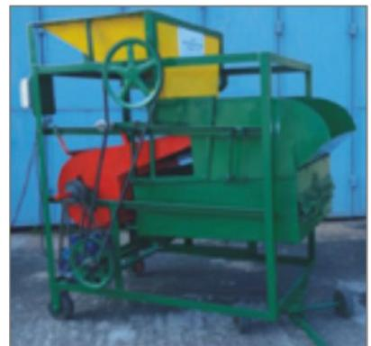
**CRRRI Mini Paddy Parboiling Unit** is a small size parboiling unit to produce quality parboiled rice by employing improved process. The process involves soaking the paddy at 75 OC for 3.5 hrs followed by open steaming for 30-45 minutes. The process ensures uniform parboiling, without any bad smell and produces light coloured rice with better consumer preference. It takes 5-6 hours to parboil 75 kg of paddy in one batch. Cost of the machine is Rs. 5,500.
