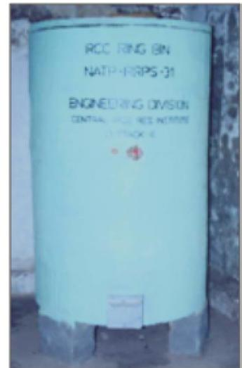
**CRRRI Chaff and Husk Stove** uses 1.2 kg of dry husk and burns continuously for 40 minutes on gasification principle. Cost of the stove is Rs. 550.
