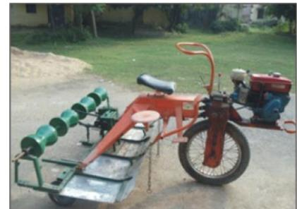
**CRRRI four row manual rice transplanter** is suitable for transplanting of 20-25 days old mat type rice seedlings. Row to row spacing is kept 24 cm. Its field capacity is 0.018-0.020 hectare per hour. It saves about 30-40% labour requirement and 40% cost in transplanting operation. Its unit cost is Rs. 8500.
