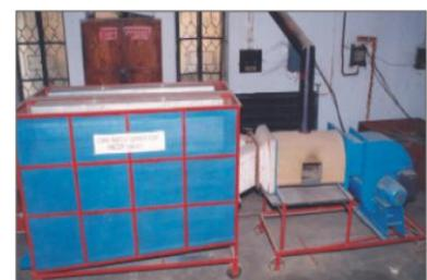
**CRRRI Community Grain Dryer** is a one ton capacity re-circulating type grain dryer using husk fired furnace. A portion of heat was supplemented as solar energy from the black painted tin roof top. Freshly harvested paddy from 24% moisture content could be dried up to 14% in 6.5 hours. Cost of the dryer without shed costs around 2.5 lakhs.
