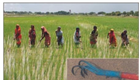
**CRRRI Star-Cono-Weeder** is suitable for weed cutting, churning and mulching in wet land. Its width of cut is 10-15 cm. It covers one row. The stars and conical drums cut the weeds and churn them into the soil. It reduced labour requirement by 50- 75% and was found to be ergonomically suitable for local labour. Its field capacity is 0.013-0.017 hectare per hour. Its unit cost is Rs. 1850.
