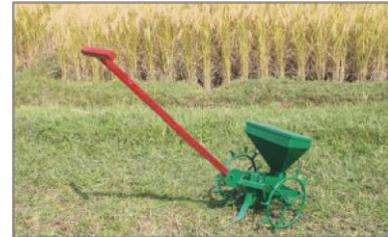
**CRR I two row manual seed drill** is a manually pulled seed drill. It consists of frame, seed box, 2 cup metering wheels with ten cups in wheels, one axle, two ground wheels, float and two furrow openers are fitted in the frame for dry sowing. It is suitable for dry sowing of paddy seed at row spacing of 20 cm. It has cup type seed metering mechanism. Its field capacity is 0.019 to 0.022 hectare per hour. Its unit cost is Rs. 3000.
