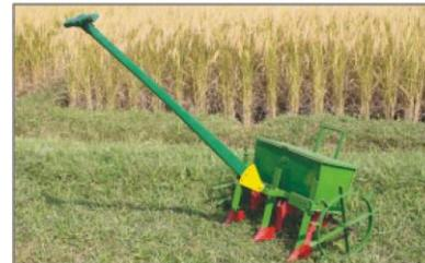
**CRR I Bullock drawn three row seed drill** is a three row seed drill having cup type seed metering mechanism pulled by a pair of bullock. It is suitable for sowing rice in dry field. Its field capacity is 0.15 hectare per hour. Its unit cost is Rs. 8000.
