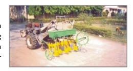
**CRRI Power tiller operated seed drill for rice and Groundnut** is a five row seed drill having plastic wheels with grooves on its periphery as seed metering mechanism. It is suitable for dry sowing rice and groundnut. Its row to row spacing is 25 cm. The cost of the seed drill is Rs. 22,000. The field capacity of 0.14 and 0.15 hectare per hour and cost of planting of Rs. 1240 per hectare and Rs. 1200 per hectare was observed for rice and groundnut, respectively.
