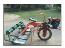
**CRRI** four row manual rice transplanter is suitable for transplanting of 20-25 days old mat type rice seedlings. Row to row spacing is kept 24 cm. Its field capacity is 0.018-0.020 hectare per hour. It saves about 30-40% labour requirement and 40% cost in transplanting operation. Its unit cost is Rs. 8500.
