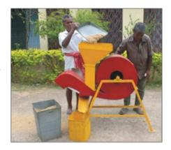
**CRRI Power Rice Winnower cum Cleaner** is a power operated machine to clean threshed paddy crop. Its capacity is 500 kg/hr of clean paddy, having cleaning efficiency of 99%. Cost of the machine is Rs.1 8,000.
