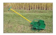
**CRRI Three row manual paddy seed drill** has fluted roller type seed metering mechanism. It is suitable for dry sowing of paddy seed at row spacing of 20 cm. Its field capacity is 0.03-0.04 hectare per hour. Its unit cost is Rs. 4000. The machine saved seed and labours in sowing of crops along the rows that helped in weeding and interculture operation.
