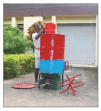
**CRRI Mechanical Rice Dryer** is a variable capacity batch dryer of 125-500 kg capacity. Both raw and parboiled paddy can be dried in this dryer. Drying is accomplished on thin layer principle. The air temperature can be maintained at  $40 \pm 2$  OC throughout the drying period. Paddy at moisture content of 20% was dried to 14% in 6-7 hrs using 10 kg of coal in the furnace. Cost of the dryer is Rs. 50,000.
