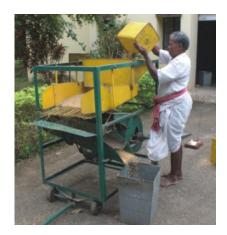
**CRRI Power Rice Seed Cleaner** is a power operated machine to clean threshed paddy crop for seed purpose. Its capacity is around 8 q/hr of clean paddy, having cleaning efficiency of 99%. Cost of the machine is Rs. 30,000.
