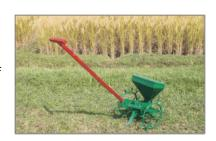
**CRRI two row manual seed drill** is a manually pulled seed drill. It consists of frame, seed box, 2 cup metering wheels with ten cups in wheels, one axle, two ground wheels, float and two furrow openers are fitted in the frame for dry sowing. It is suitable for dry sowing of paddy seed at row spacing of 20 cm. It has cup type seed metering mechanism. Its field capacity is 0.019 to 0.022 hectare per hour. Its unit cost is Rs. 3000.
