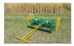
**CRRI Six row manual drum seeder (Cylindrical shape)** is suitable for sowing of sprouted paddy seed in puddled field at row spacing of 20 cm. Its field capacity is 0.037-0.04 hectare per hour. Its unit cost is Rs. 6500. It reduced seed rate by 35-40% as compared to broadcast seeding and reduced weeding cost about 55%.
