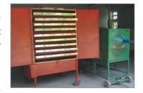
**CRRI Domestic Solar Dryer** is a cabinet type domestic solar dryer to dry 0.5 - 1 kg food material. The dryer is rectangular in shape. The top glazing is of 4 mm plane glass. The dryer is placed on a stand inclined at an angle of 300 to the horizontal. A sliding type loading tray enters from the top end of the dryer. Cost of the dryer is Rs. 1,500.
