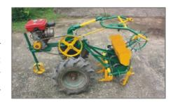
**CRRI Power tiller operated seed drill for rice and pulse** is a five row seed drill having fluted roller type seed metering mechanism. It is suitable for dry sowing of rice, wheat, green gram, and black gram etc. Its field capacity is 0.14 hectare per hour. Its unit cost is Rs. 20,000.
