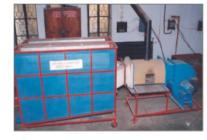
**CRRI Community Grain Dryer** is a one ton capacity re-circulating type grain dryer using husk fired furnace. A portion of heat was supplemented as solar energy from the black painted tin roof top. Freshly harvested paddy from 24% moisture content could be dried up to 14% in 6.5 hours. Cost of the dryer without shed costs around 2.5 lakhs.
