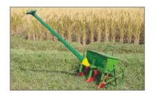
**CRRI Bullock drawn three row seed drill** is a three row seed drill having cup type seed metering mechanism pulled by a pair of bullock. It is suitable for sowing rice in dry field. Its field capacity is 0.15 hectare per hour. Its unit cost is Rs. 8000.
