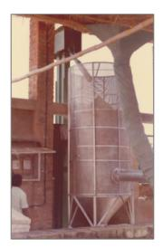
CRRI Solar and Bio Mass Fired Multi Crop Dryer is a batch dryer of 300 kg paddy holding capacity. Its
