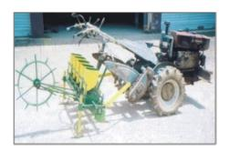
**CRRI Ten row tractor drawn seed drill** is a ten row seed drill and suitable for seeding in dry field. The field capacity of the seed drill is 0.8 hectare per hour. Row to row distance can be adjusted. The unit cost of machine is Rs. 50000. It saved 70% time and 55% labour cost and weeding cost as compared to broadcasting and transplanting method.
